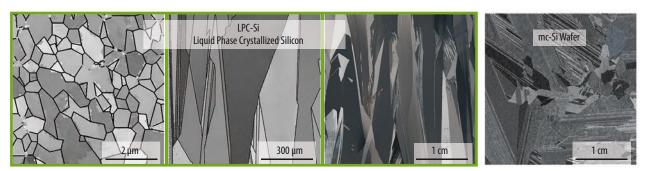
Fig. 3 The green box depicts the flexible grain size tuning achieved with the LPC technology utilizing a line-shaped diode laser. Depending on the crystallization parameters, the grain size ranges across several orders of magnitude and can be tuned to fit the desired requirements (left). A micrograph of a multi-crystalline Si (mc-Si) wafer is depicted in the grey box for comparison (right; Source: HZB / HySprint).
