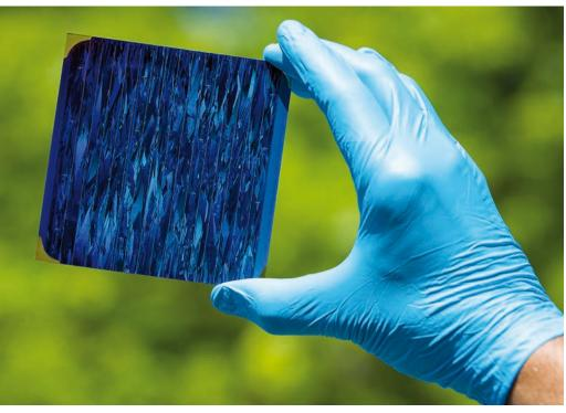
Fig. 4 Si crystal grain structure created by cw line shaped diode laser LPC treatment of a 10  $\mu$ m Si thin film on 10 cm  $\times$  10 cm glass substrate. (Source: HZB / HySprint)
