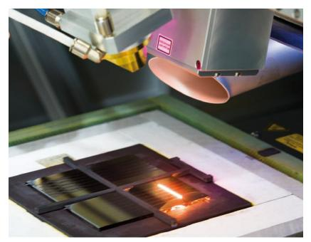
Fig. 1 Line-shaped continuous-wave laser crystallization of a 10  $\mu$ m thin silicon film on a 3 mm thick glass substrate (Source: HZB / HySprint)
