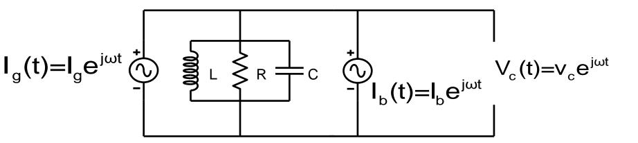
• Beam and RF generator are represented by a current source
