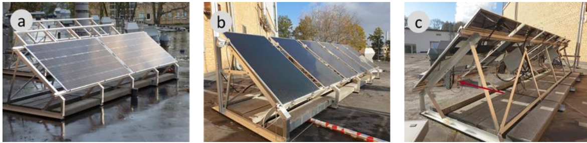
Figure 10: Integration of the PV modules (a) the SHJ/HJT modules from Enel Green Power and (b) the CuInGaSe thin film PV modules from Solibro Research AB installed at the test site of FZJ. As an example, a photograph (c) showing the PEM electrolyser (indicated by the arrow) directly mounted onto the back of one of the CuInGaSe thin film PV modules in the so-called cassette design.
