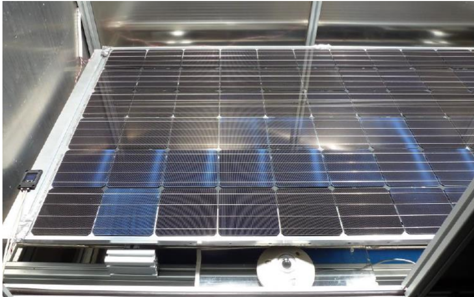
Figure 4: PV module in the sun simulator at FZJ. The radiation intensity of the sun simulator is monitored using a monitor cell which is visible at close to the bottom left hand corner of the PV module and a pyranometer visible at the centre of the bottom edge of the photograph.
