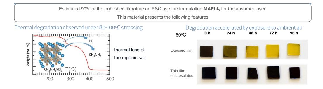
By tuning the AB and X stoichiometry (ABX<sub>3</sub>) of the perovskite, OxPV has developed a perovskite with improved thermal stability
