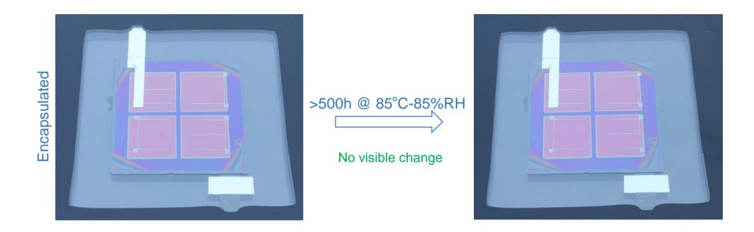
Scalable encapsulation process compatible with standard module assembly process
