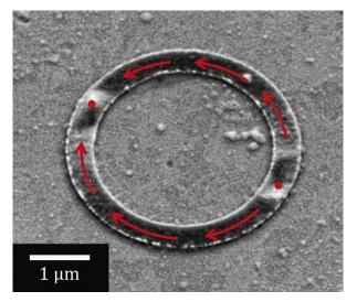
Scanning electron micrograph of a ferromagnetic ring that exhibits magnetisation (black & white contrast) along the ring and forms two domain walls.
