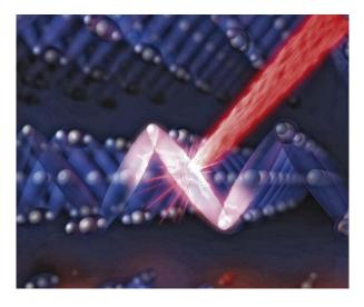
An optical laser flash (red) disrupts the electronic order (blue) in magnetite, switching the material's state from insulating to conducting within a trillionth of a second.
