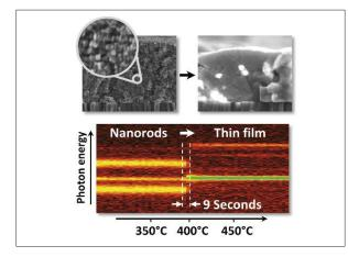
The transition from a layer of densely packed nanorods (top left) into a polycrystalline semiconductor thin film (top right) can be observed in realtime using in-situ X-ray diffraction. In the bottom image, the intensity of the X-ray signals is colour-coded. Detailed analysis of the signals reveals that the transformation from nanorods to kesterite crystals takes only 9 to 18 seconds.
