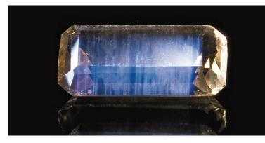
Blue sanidine variety. After a while, the crystals display defects that can be "healed" with high temperatures. HZB researcher Johannes Kähn investigated exactly what happens during the process.
