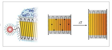
A water-soluble Ni(II) catalyst allows the polymerization of ethylene in aqueous solution. The illustration shows how the newly created parts of the PE chain are incorporated into the growing crystal. The amorphous areas act in the ideal nanocrystal like deflection pulleys that reverse the direction of the chains by 180 degrees.
