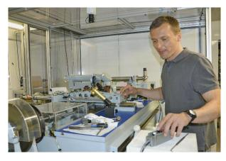
The sawtooth structures are created in this machine. A diamond rules the tiniest of grooves into the gold-coated silicon substrate.
