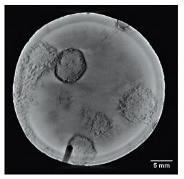
2D X-ray computer tomogram of the Tiberius sesterce taken from the collection in the Duke Anton Ulrich Museum in Braunschweig. Shown is the core of the coin with the drilled hole hailing from an earlier analysis (bottom left) as well as two points of zinc depletion (round surfaces).
