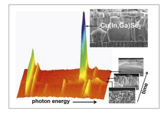
Growth of the layers can be analysed using in-situ X-ray scattering and fluorescence signals.
