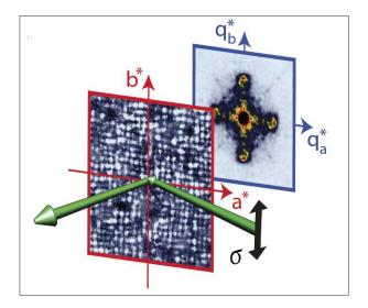
Stripe pattern of charge carriers in  $Bi_2Sr_2CaCu_2O_{8+x}$ . The figure shows the structure with a period of about one nanometre (front) and the associated diffraction pattern (back) in the form of a so-called Fourier transformation.
