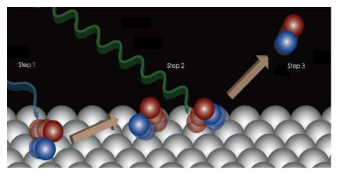
First, the CO molecules were detached from the crystalline surface of the ruthenium catalyst using conventional laser pulses (blue), after which the researchers could observe using X-ray pulses on the LCLS (green) that these molecules remain close to the surface over a substantial period of time and can only move parallel to it. Only after a certain time (step 3) do the CO molecules completely escape from the surface.
