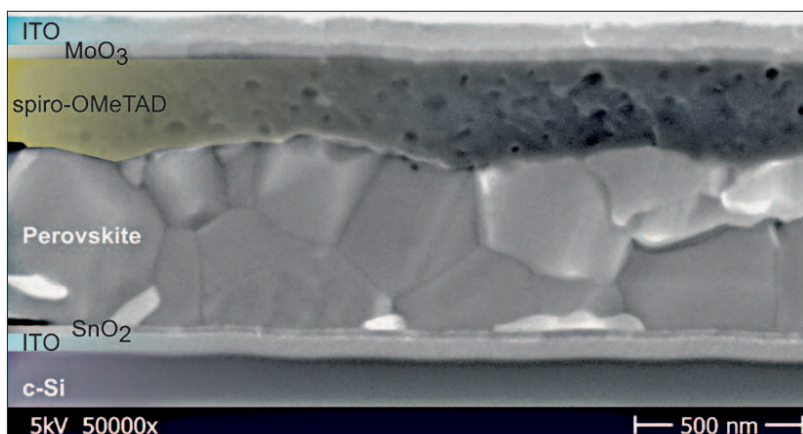
Schematic structure of the silicon-perovskite hybrid tandem cell.
