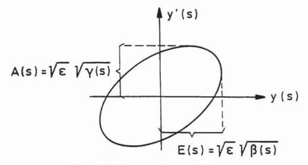
Figure 27: Beam envelope and divergence
