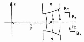
Figure 4: Shape of magnetic field around design orbit
