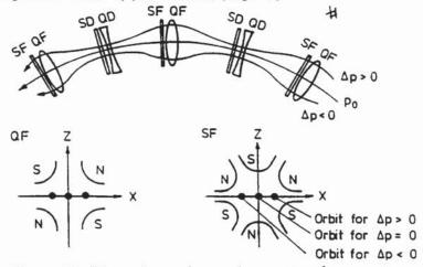
Figure 35: Dispersion trajectory in a sextupole magnet
