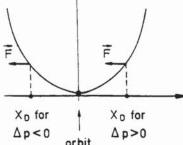
Figure 36: Force on electrons in a sextupole magnet
