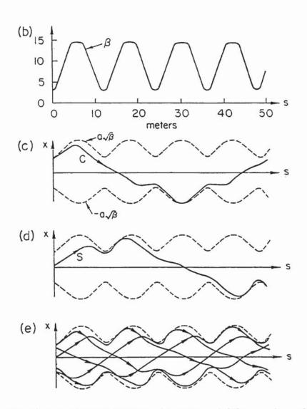
Figure 28: a) A regular FODO lattice of focusing and defocusing lenses b) Beta-function. c) Cosine-like trajectory for s=0. d) Sine-like trajectory for s=0. e) One trajectory on several successive revolutions. (According to M. Sands, The Physic of Electron Storage Rings, SLAC-121).
