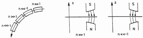
Figure 5: Alternating-gradient focusing
