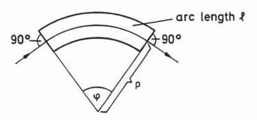
Figure 19: Dipole sector magnet
